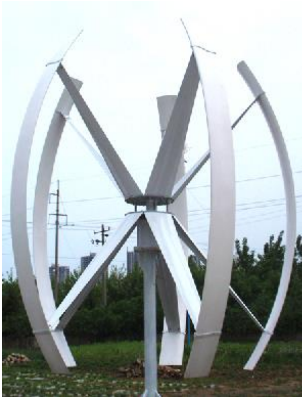
Figure 16 - Vertical wind turbine VAWT , helical vertical wind turbine
