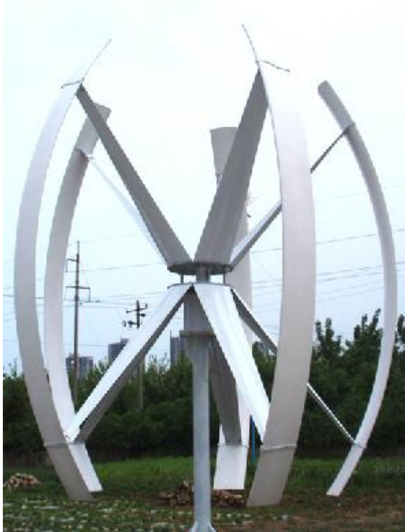
Figure 17 - Vertical wind turbine VAWT , helical vertical wind turbine
