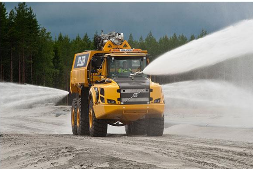
Figure 15 Unifire’s unique F50-ST Side Turret
